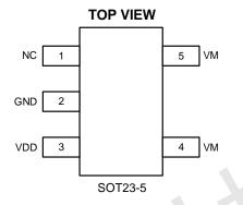
Figure 2. Pin Configuration
